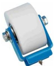
The KIT is made up by a painted steel fork with idle rollerset. The polyamide rollerset is installed on greased bearings. Operating temperature of the rollerset  $< 80^{\circ}\text{C}$ . Please specify the positioning (**H** or **Y**), otherwise it will be supplied with **H** execution. Executions with dimensions and profiles on request (1,2,3,4).
