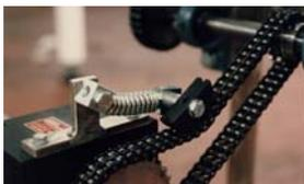
Then came ARCO, an elastic rotating element completely made of steel, compact and that can work in very heavy conditions as low and high temperatures.
