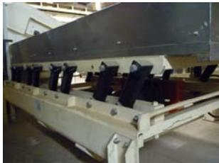
CRESA, VIB and CIAO are three range of products that exploit the same functional principle, that is the elastic deformation of four rubber cylinders, lodged inside the hollows resulting from the coupling of two square-section elements rotated 45° with respect to each other. CRESA made of steel and CIAO, made of plastic, are essentially elastic rotating elements that are prevalently used as automatic chain tightener and belt tightener, equipped with the relative specific kits.
